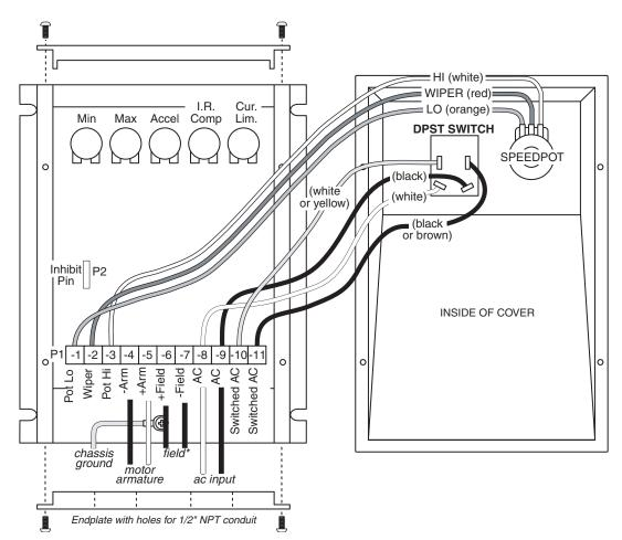
\* Used for shunt wound motors only! No connection is made to these terminals when using permanent magnet motors.
