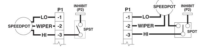
NOTE: Permits starting and stopping of motor without breaking AC lines. In the event of SCR failure or false triggering, the Inhibit circuit will not stop motor.
