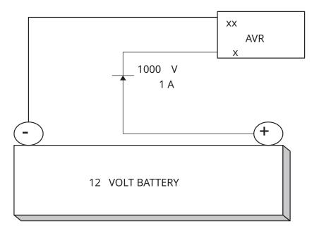
**NOTE:** If the generator set battery is used for field flashing, the generator main stator neutral must be disconnected from ground.
