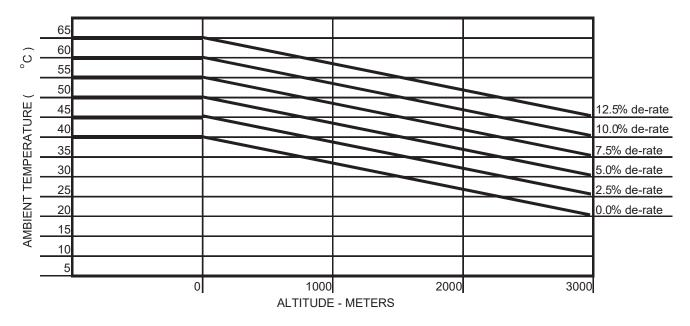
Altitude & High Ambient Temperature Operations – For applications over 1000 meters (3300 feet) elevation or where the temperature of the ventilating air to the generator exceeds 40°C (104°F), derating of the generator is necessary.
