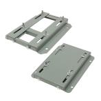
and painless motor positioning. All D Bolts (motor mounting bolts) are Grade 5 for strength, welded into position to prevent spinning and "dropping" from slots, and fixed to the exact foot pattern of the motor to aid in easier motor installation.
